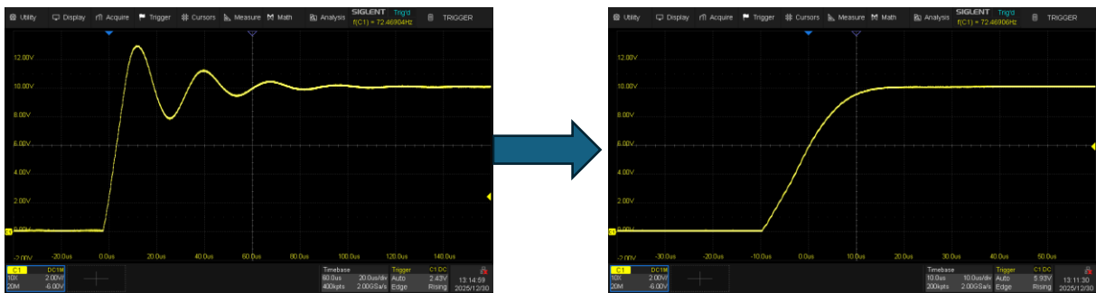
Waveforms Comparison Before and After APFC Adjustment
