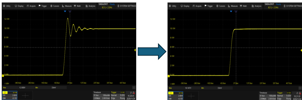
Waveforms Comparison Before and After APFC Adjustment
